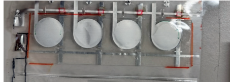
Fig 2: A spray-coated super-capacitor operating @ 3.2 V
