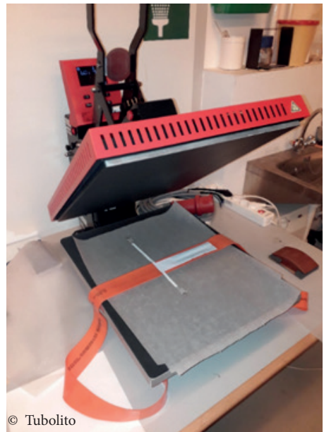
Figure 6: Hot press lamination of sensors on bicycle tube
