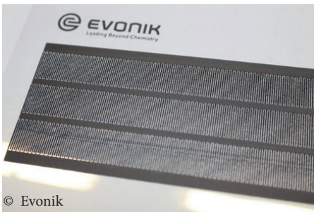
Figure 5: serial arrangement of 3 cells in coplanar design
