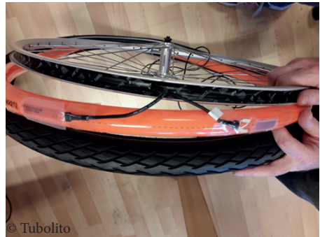
Figure 8: First preliminary version of the SYMPHONY demonstrator for the pressure measurement in bicycle tubes
